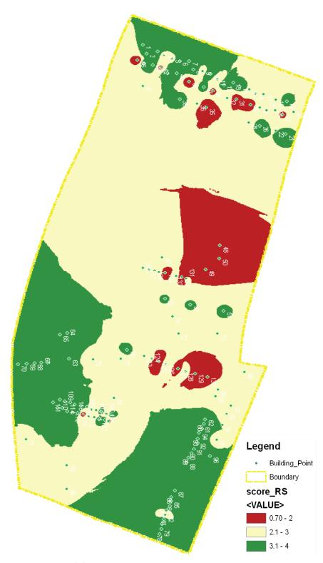
Fig. 2: RVS Score by desk study using high resolution satellite data
